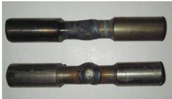
Fig 1: Comparison of MIG and TIG welding Specimens
